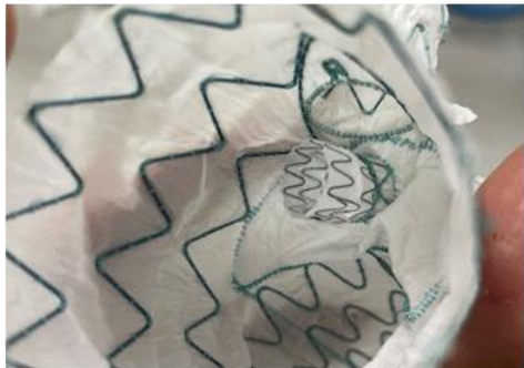
Case 1: 5mm inner tunnels Average force 4.71N
