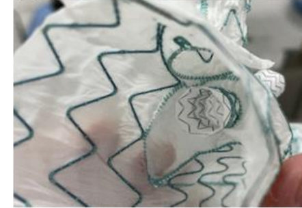
Case 3: BE stent with flare Average force 8.09N
