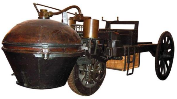
Nicolas Cugnot (1770) Steam engine Maximum speed 2mph
